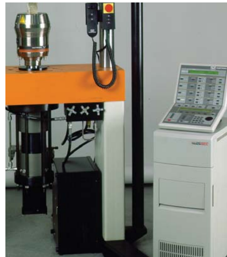
▲ A 1340 frame, upgraded with a FastTrack 8800 tower controller
