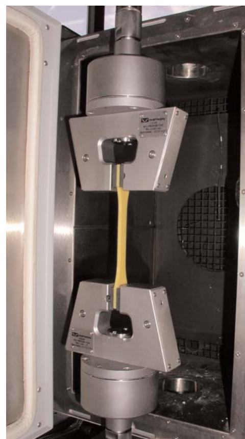
▲ Pneumatic high-temperature grips inside a chamber
